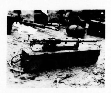
33. Electrically fired .256 calibre sub-calibre rifle found in BALIKPAPAN.
